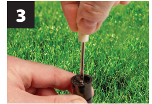
3 Distance Adjustment Turn screw clockwise to reduce up to 25%.
